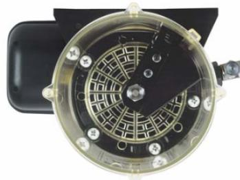
The gear motor is protected by means of an IP-56 protection degree covering (NYLON PA6). The seal is guaranteed from well-mounted "o"-ring. The pumps can have an integrated electronic control timer (1) built into the covering. The timer can be preprogrammed to automatically operate the pump with variable "run" and "pause times".
